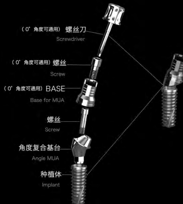
角度复合基台装配示意 Steps to place angled MUA
